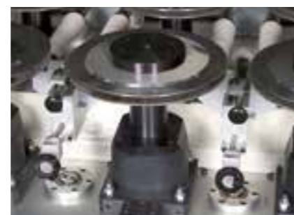
Additional adjustable rollers to support the profiles with particular shapes.
